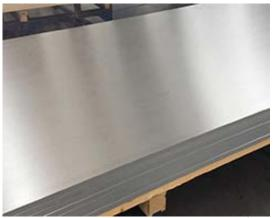
with enamel, which is suitable for building decoration materials. It contains a small amount of Cu, so its strength is higher than that of 6063, but its quenching sensitivity is also higher than that of 6063. Air quenching cannot be achieved after extrusion, and it needs re-solution treatment and quenching aging to obtain higher strength.
