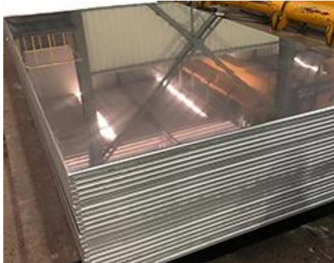
aluminum is about 20% higher than 5052; Its characteristics are similar to 5154, but the corrosion resistance of 5454 aluminum plate is better than 5154 aluminum plate in severe environment. Therefore, 5454 aluminum sheet is generally used in environments with high anti-rust requirements, such as marine facility pipelines, aluminum tank trucks bodies, car wheels, etc.
