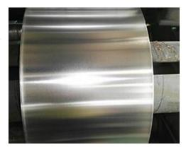
plasticity is still good when semi-cold hardening. Low plasticity, good corrosion resistance and good weldability when cold work hardened, but poor machinability.
